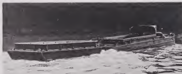
FIGURE 13. Loaded 2\frac{1}{2} -ton amphibious trailer towing astern of loaded DUKW.
